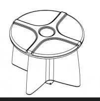
Set product into required position and mark off the centre of each position to be drilled through the fixing plate
